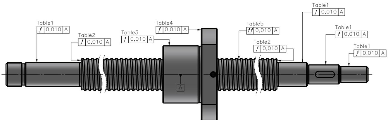
Table 2: Radial run-out bearing seat related to the centerline of screw groove and radial run-out of journal diameter related to the bearing seat.
