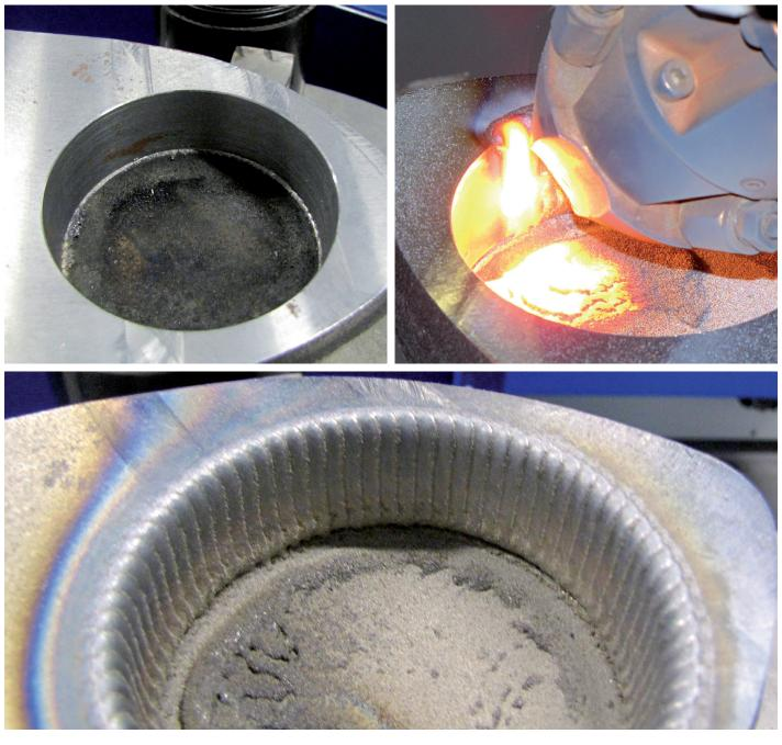
Surface cladding can be carried out on outer and inner diameters.
