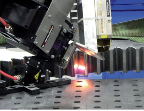
We can harden sides of toothing from a module of 4 mm.
