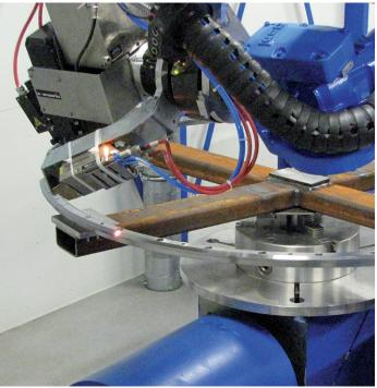
We are able to harden rotary parts of large diameters.
