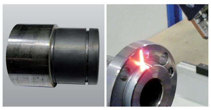
Due to thee scanning technology is the temperature controlled locally, which ensures optimal hardening temperature and prevents partial melting of edges.
