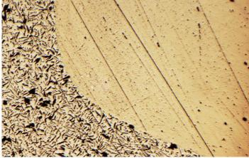
Arc welding using E-S716 electrode (50%Ni), 4 layers, calking and brushing of each layer; waiting for the cooling of each layer – about 40 min.
