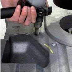
Preparing for weld by drilling
