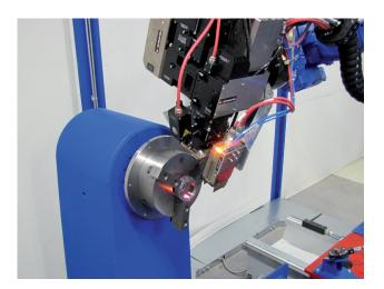
Laser tempering uses the self-cooling effect of the material to create the tempered layers.
