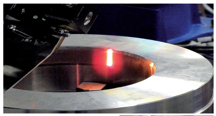
With scanning and focusing of the beam at a distance of 170 mm from the front of the head, we are able to harden cavities with the depth distance of up to 140 mm.
