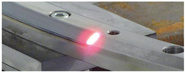
We can make laser hardenning on supporting elements of machine tools.
